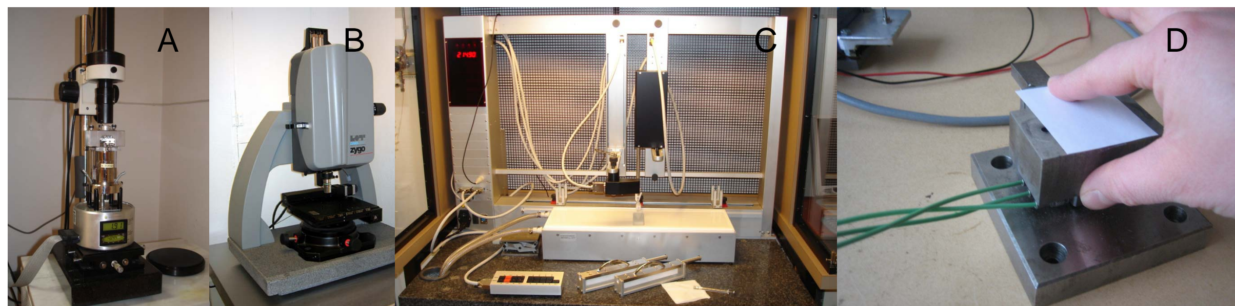
Figure 1: A) An Atomic Force Microscope (AFM), used for imaging and friction measurements on model surfaces B) Profilometer, used for measuring topography and surface roughness C) Langmuir-Blodgett, used for deposition of silica particles to produce model surfaces D) A macroscopic friction device, used to measure friction between a human finger and different surfaces.
